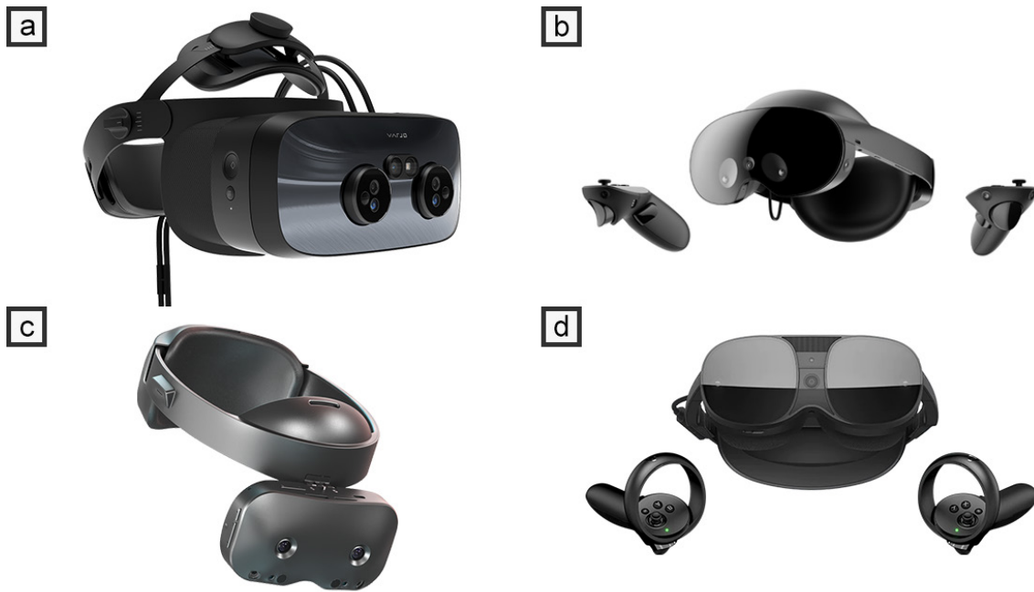
Figure 16 – (a) Varjo XR-3 (released 2021) is a tethered MR device with marker-based tracking and 6-DoF via a beta. (b) Meta Quest Pro (released 2022) with MR support via 6-DoF tracking (5 cameras) and colour passthrough. (c) Lynx R-1 (released 2022) focuses primarily on AR but can support VR with 6-DoF tracking via 2 cameras and colour passthrough. (d) HTC Vive XR Elite (released 2023) with MR support via 6-DoF tracking with 4 cameras and colour passthrough.
