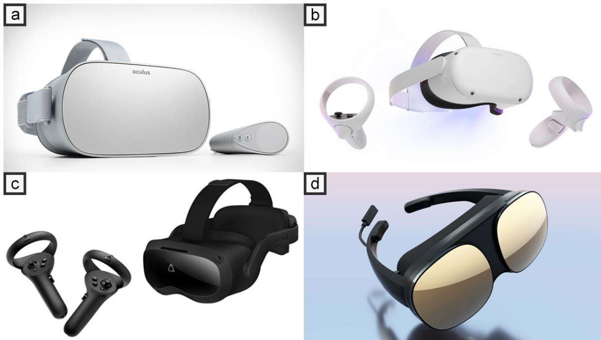
Figure 15 - (a) Oculus Go (released 2018) with only 3-DoF tracking. (b) Meta (formerly Oculus) Quest 2 (released 2020) with 6-DoF tracking and grayscale passthrough. (c) HTC Vive Focus 3 (released 2021) with 6-DoF tracking and grayscale passthrough. (d) HTC Vive Flow (released 2021) with 6-DoF tracking and is controlled via a smartphone or remote and is meant to be linked to a smartphone.
