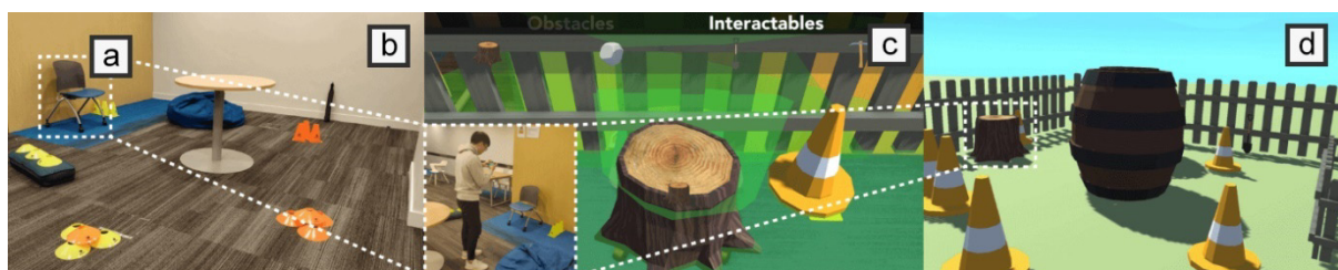
Figure 42 - ARchitect supports SR level creation in AR. (a) The real-world location and obstacles. (b) A user editing the level using smartphone AR. (c) The user adding a tree stump in place of a chair. (d) The final game level (Lin et al, 2020).
