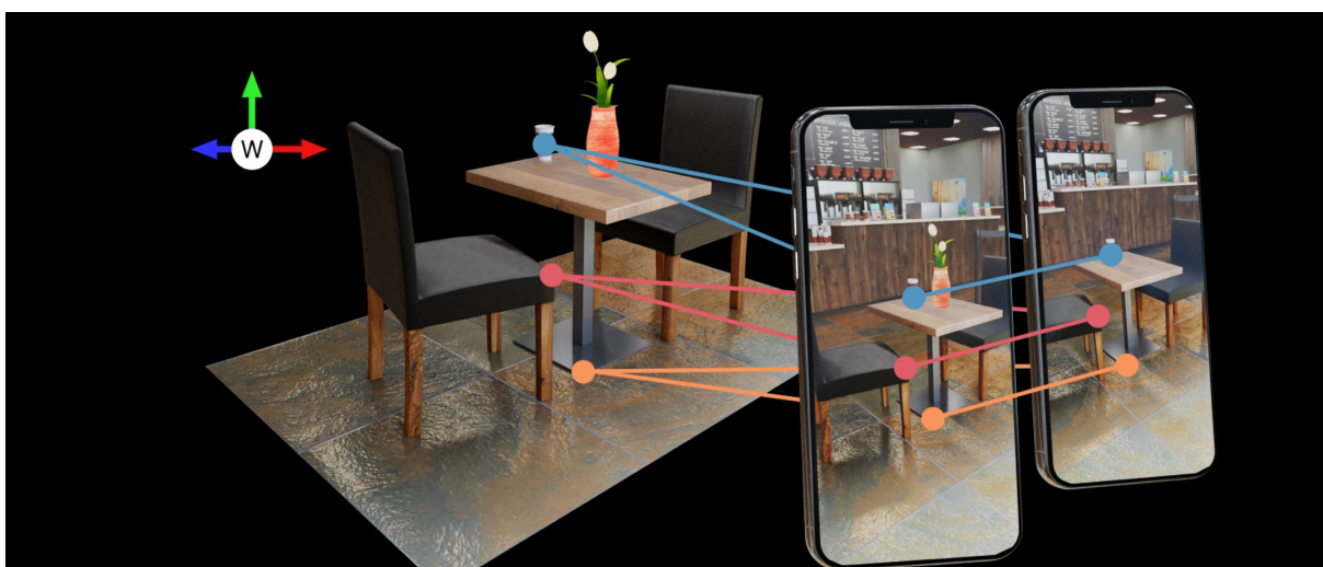
Figure 8 - Computer vision is used to track changes to points of interest (blue, red and orange dots) each frame. Changes to the device pose can be triangulated from these points and their changes over time.
