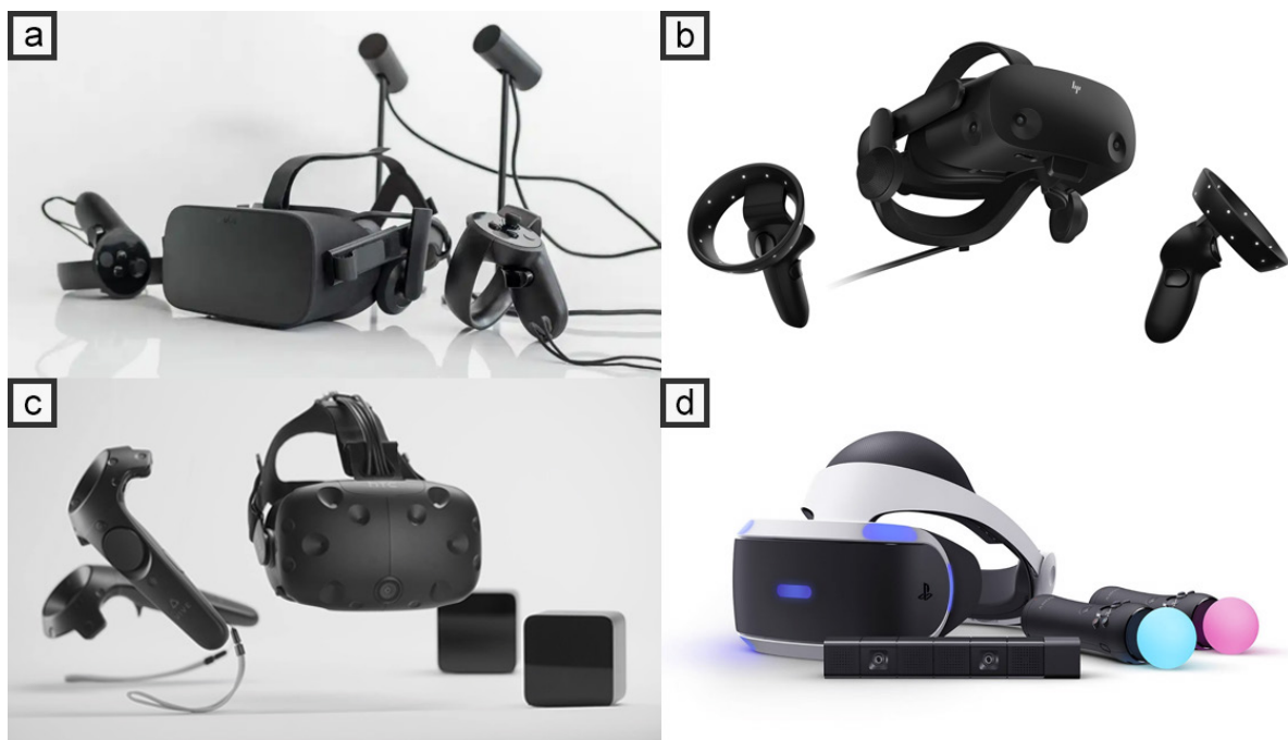
Figure 13 - (a) Oculus Quest CV1 (released 2016) with external tracking. (b) HP Reverb G2 (released 2021) with inside out tracking. (c) HTC Vive (released 2016) with external tracking. (d) PlayStation VR (released 2016) with external tracking via camera.
