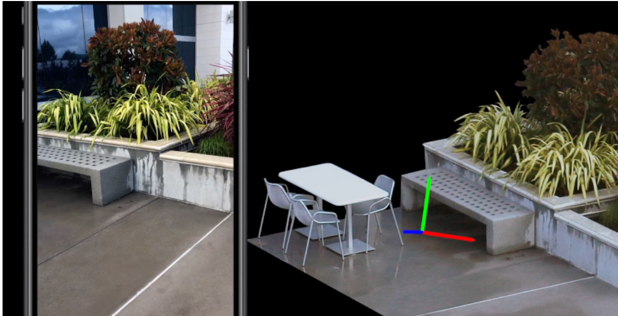
Figure 7 - Example of ARKit detecting the pose (orientation and position) of the smartphone device in the location using sensor data.
